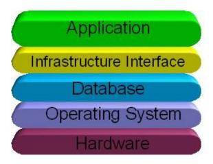
This diagram is a generalized diagram of the various tiers that make up a computer system. The Functional Requirements section discussed the Application and Database tiers and also made some comments on operating system and hardware requirements. Sometimes these functions are separated on different hardware, as discussed below.
